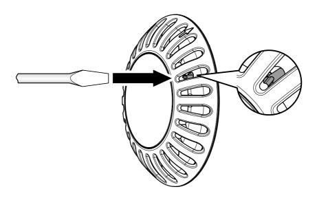
2 ROTATE ANTI-CLOCKWISE & RELEASE FROM LOCKING RING
